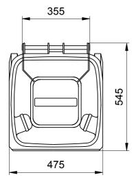
Mobile Waste Containers MGB 140 Litre Sizes, Measures, Dimensions: Hight 1050 mm; Width 475 mm; Depth 545 mm
