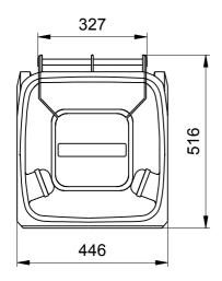
Mobile Waste Containers MGB 60 Litre Sizes, Measures, Dimensions: Hight 935 mm; Width 445 mm; Depth 520 mm
